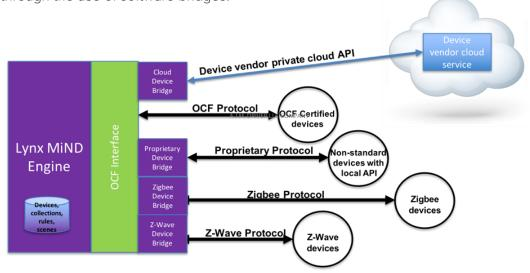
Device properties and capabilities are bridged into a common object model, where all device management activity is performed.
